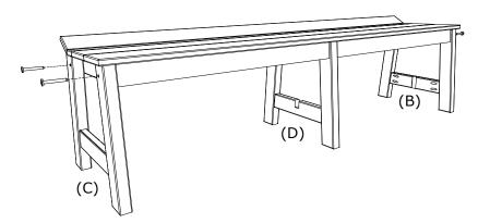
2. Attach (E) Cross Pc.to (B) (C) & (D) Leg Assemblies using 2 1 1/2" Screws per side and 1 2" Screw in center, Be sure to match all numbers & or Letters.
