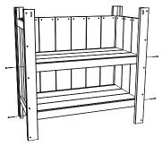
3. Place (A) Top on base keeping Placement blocks on inside of Corners, Attach remaining 4 - 2" Screws in (B) Front Panel. be sure to match all numbers & or letters.
