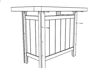
4. Attach (A) Top using 2 - 2" Screws per corner in pocket holes, be sure to match all numbers & or letters.
