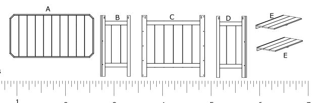
1. Attach (C) Front Panel to (B) & (D) Side Panels using 6 - 2" Screws in predrilled holes, See Notes. be sure to match all numbers & or letters.
